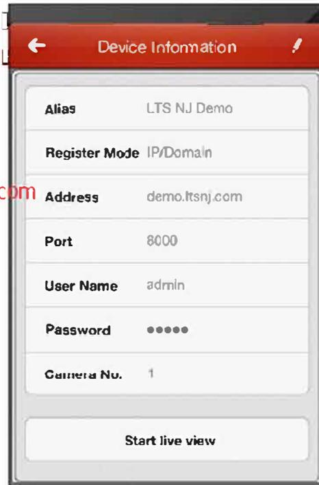
The device has been added. Tap "Start live view" to see the camera feeds. For further changes tap the pen button (✎) on the top, right corner. Tap back (←) to return to the Devices list.
